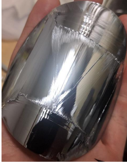
Fig. 1 Spontaneous exfoliation of a silicon thin film showing poor uniformity and surface finish.
